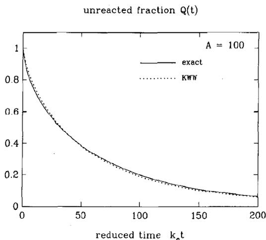
Fig. 2. Comparison of exact  $Q(t)$  with Kohlrausch-Williams-Watts function, eq. (17);  $A=100$ .
